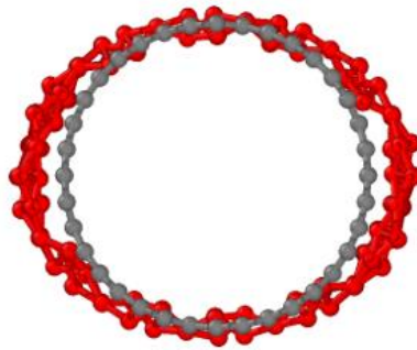
Figure 4.1 :Initial (gray) and final (red) structures of BNTs during energy minimization. \alpha -BNT is given as an example.
