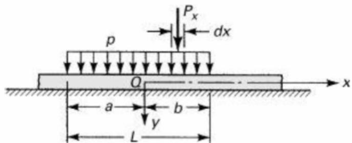
for infinite beam on an elastic foundation and loaded at the origin
